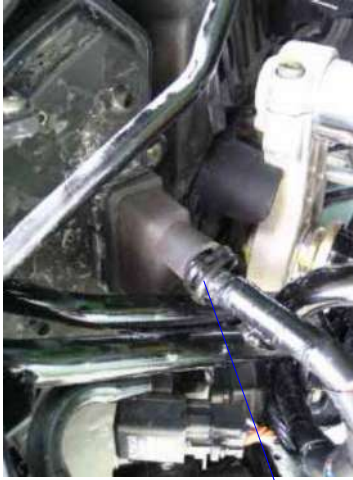
METER wire fixed hook
