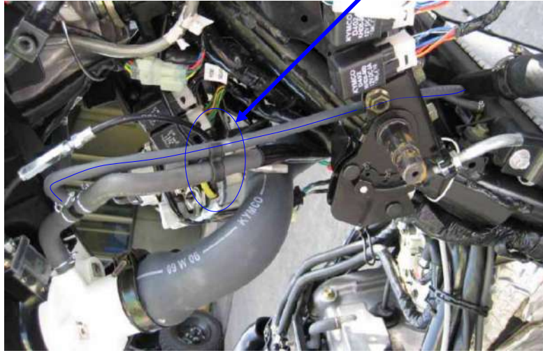
Oil gas recycle(CAP end)
