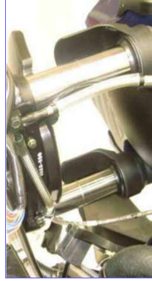
Fix position the brake oil pipe.
