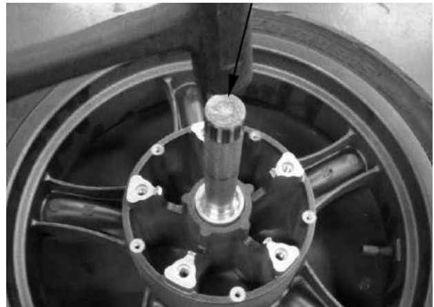
Bearing install driver
