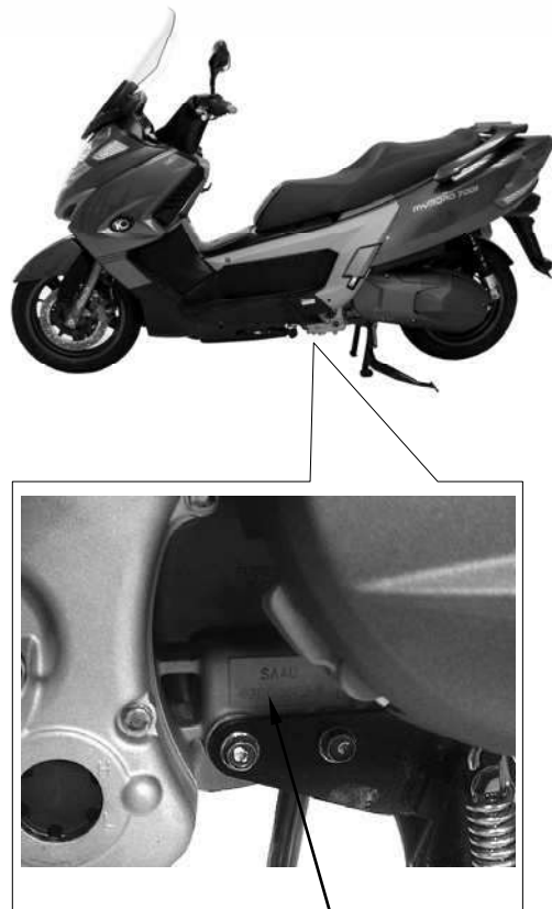
Location of Engine Serial Number
