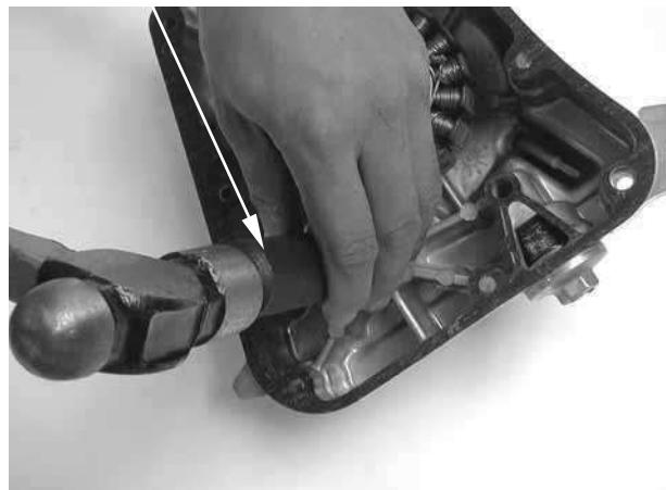
Mechanical Seal Driver
