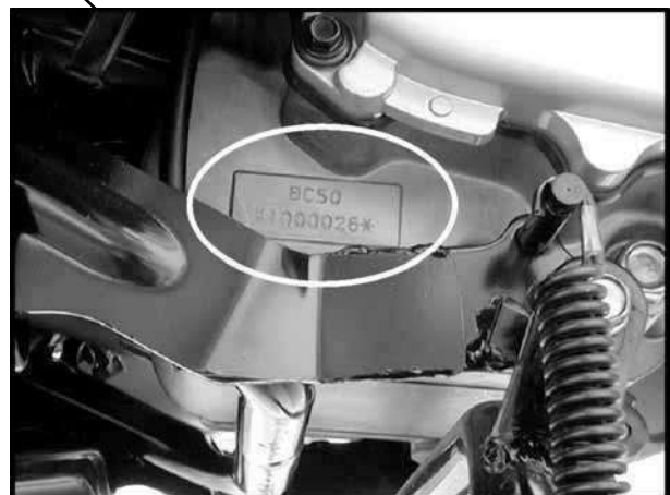
Location of Engine Serial Number
