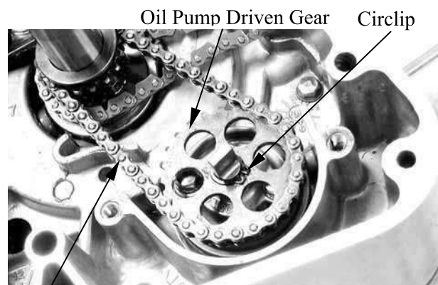
Oil Pump Drive chain
