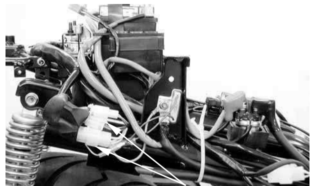
A.C. Generator Wire Connectors
