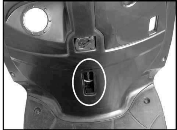
Location of Frame Serial Number
