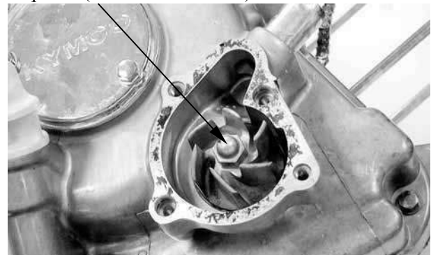
Impeller (Left Hand Threads)
