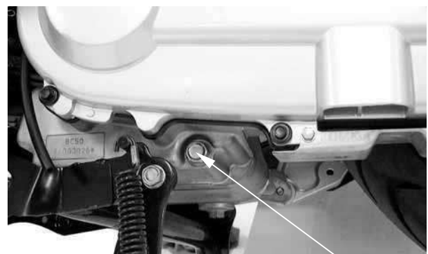
Oil Drain Bolt
