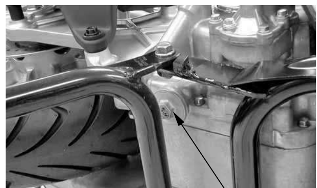
Oil Filter Screen Cap
