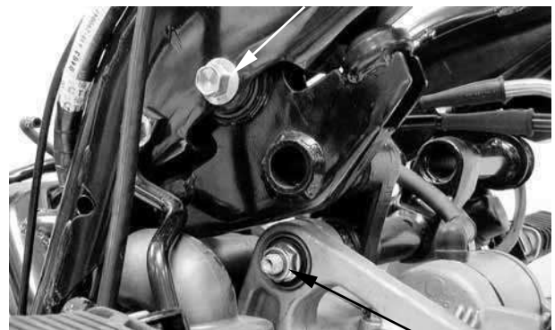
Engine Mounting Nut
