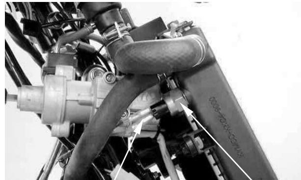
Wire Thermostatic Switch
