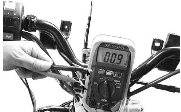
Stop Switch Wire
