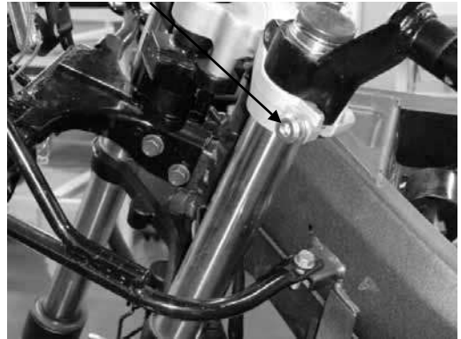
Upper Fork Bridge Bolts
