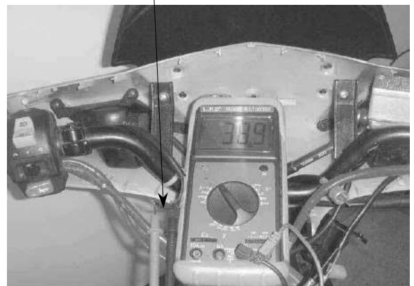
Stop Switch Wire
