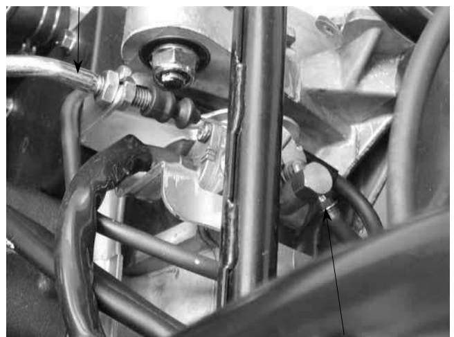
Oil Outlet Line
