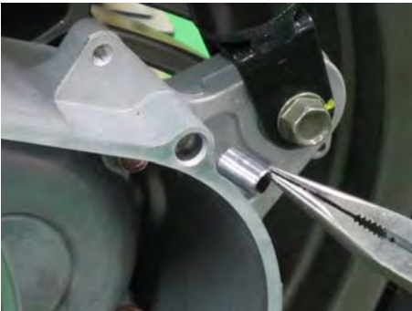
Remove the two dowel pins.
