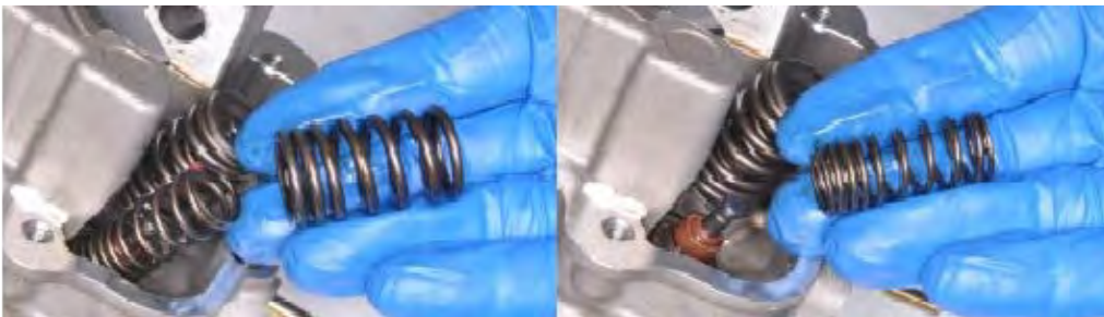
Remove the valve springs.
