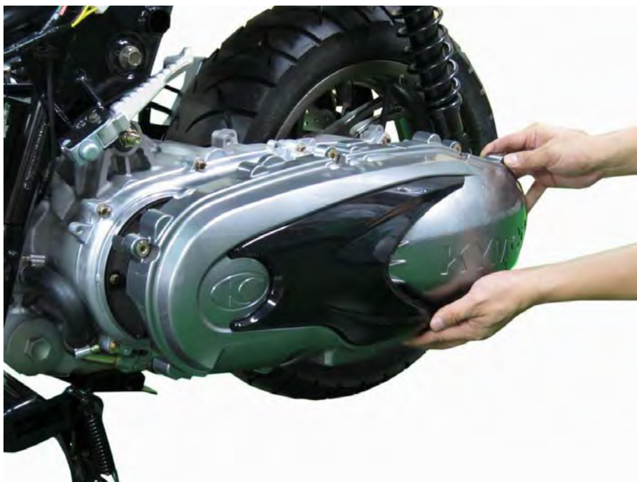
Install the belt case plastic cover.
