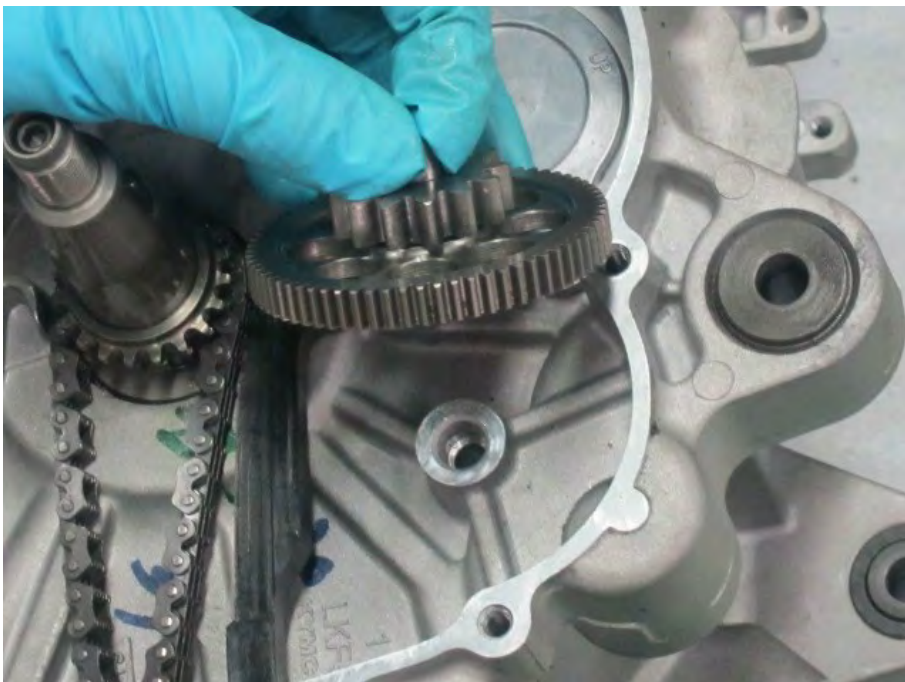
Remove the starter idle gear and shaft from the crankcase.
