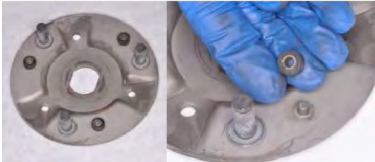
Inspect the clutch shoe bumpers and replace them as needed.
