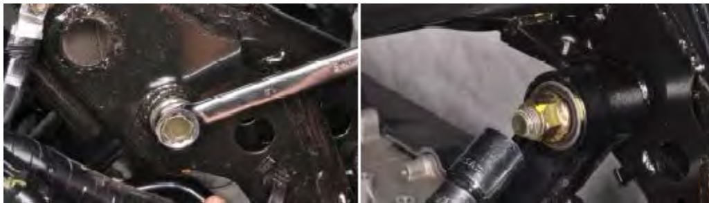
Hold the engine mounting bolts with a 14 mm wrench and torque the nuts to specification with a 19 mm socket.
