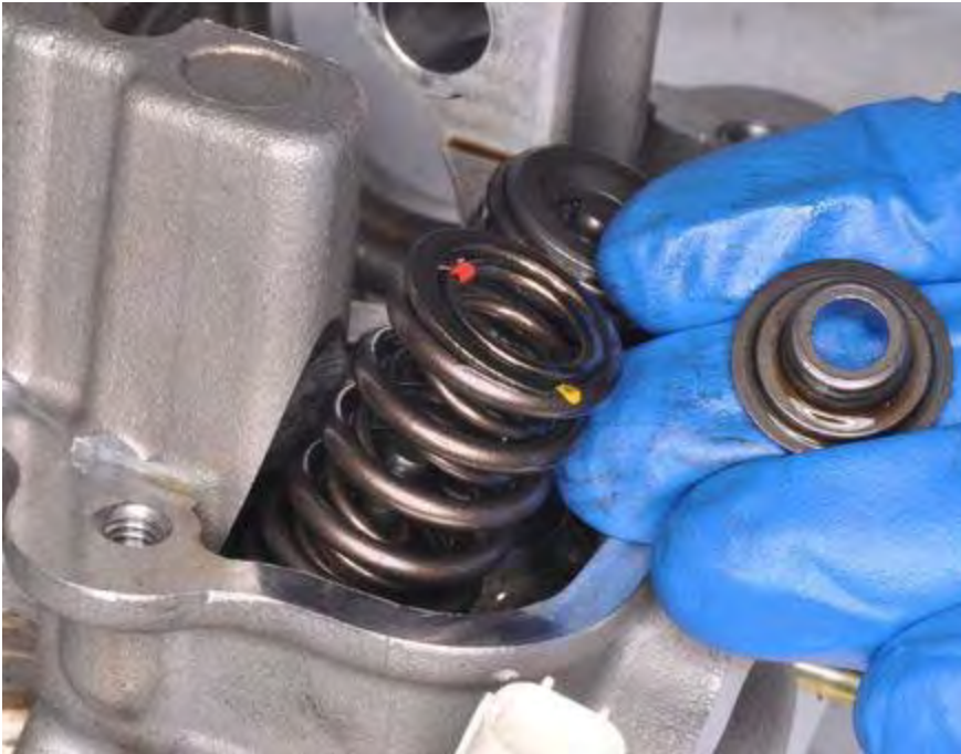
Remove the spring retainer.
