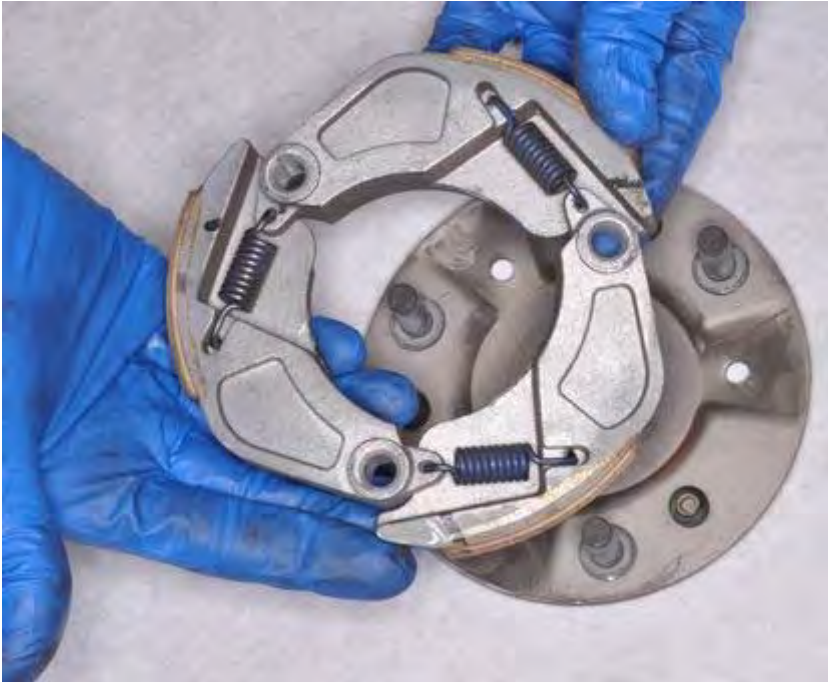
Slide the clutch shoes off of the pivots on the drive plate.
