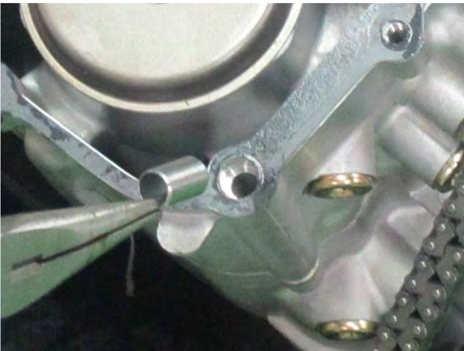
Remove the two dowel pins.
