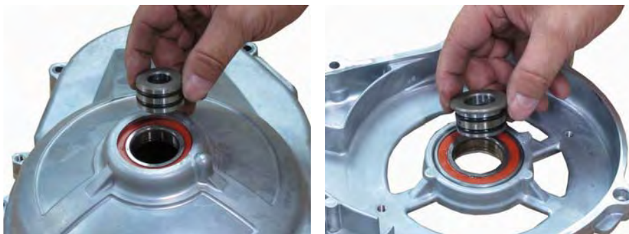
Remove two bearing collar.
