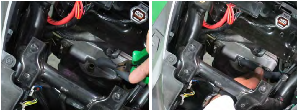
Install the breather hose to the cylinder head cover. Secure the hose with the clamp.
