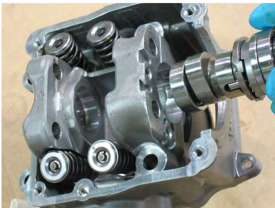
Remove the camshaft from the cylinder head.
