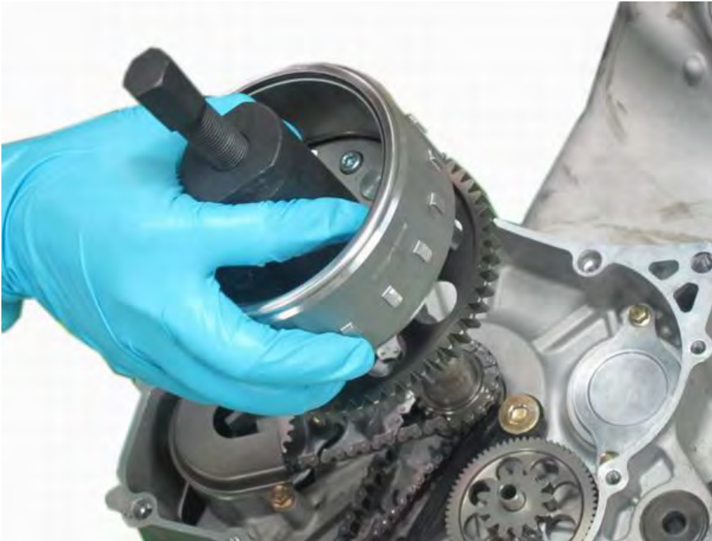
Remove the flywheel from the crankshaft.
