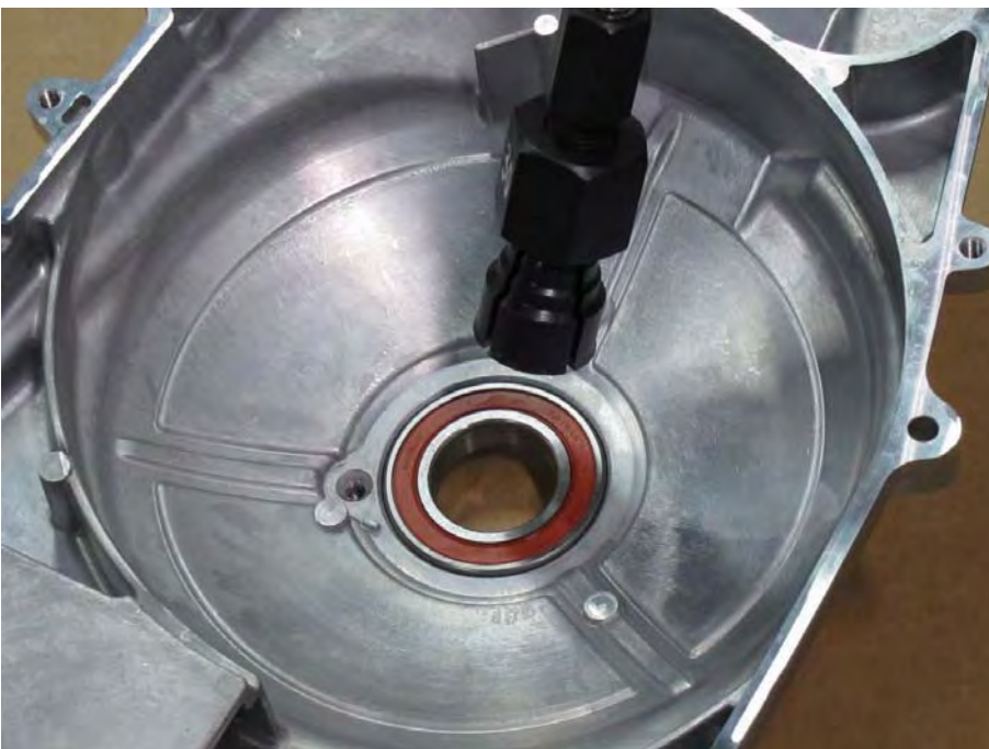
Remove the bearing with a suitable bearing puller.
