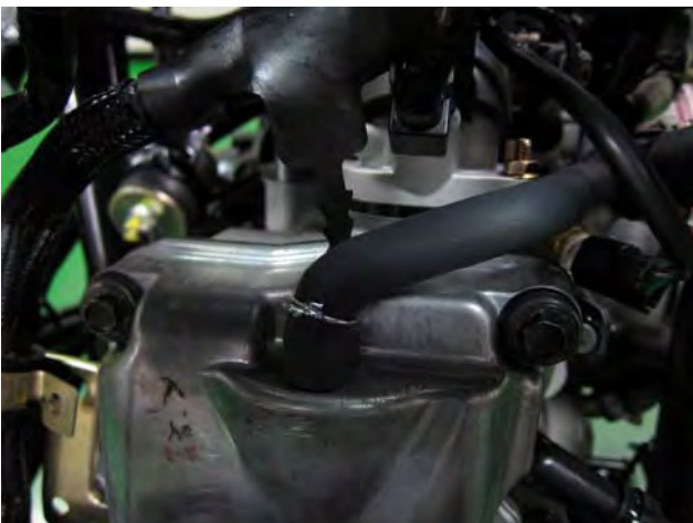
Install the breather hose to the cylinder head cover. Secure the hose with the clamp.
