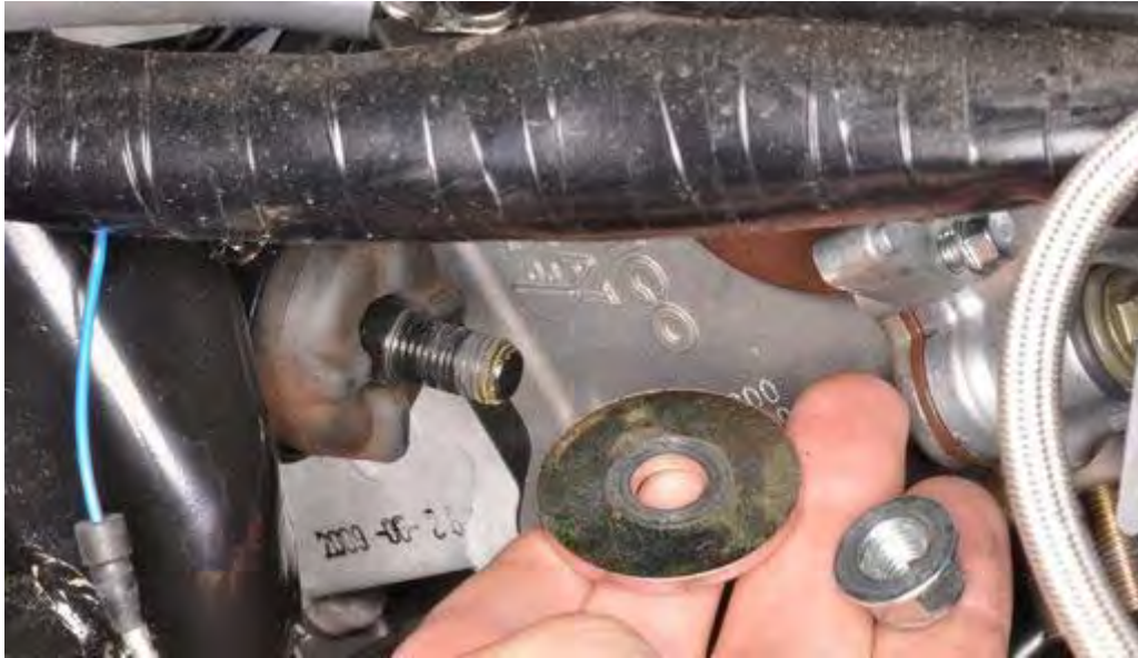
Install the engine mounting bracket damper washer and nut.
