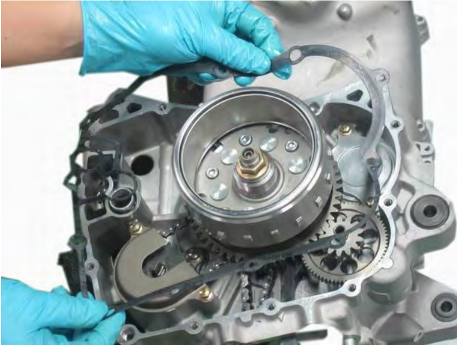
Remove the generator cover gasket.
