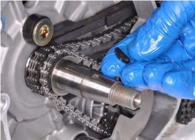
Remove the woodruff key from the crankshaft.
