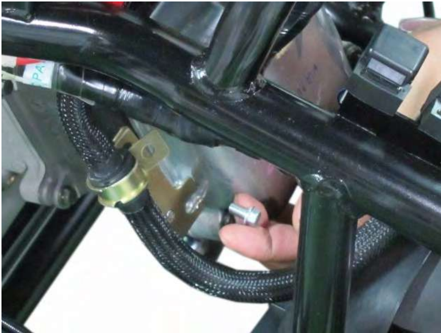
Fit the fuel stay into place. Tighten the stay bolt securely with an 8 mm socket.
