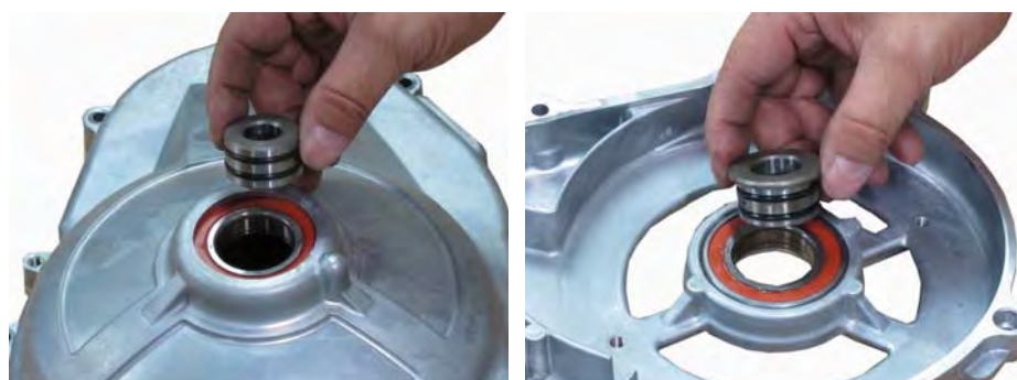
Remove two bearing collar.
