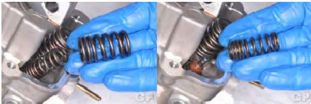
Remove the valve springs.
