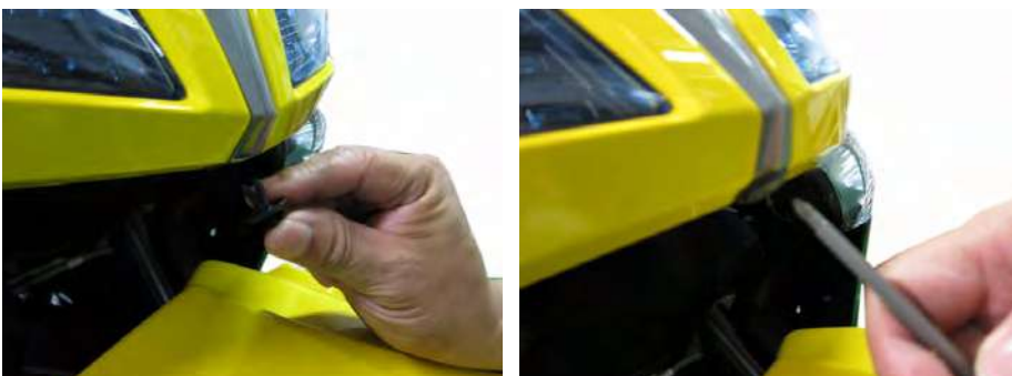
Align the two posts with the grommets. Carefully push on the small black cover. Install the small black cover push pin.
