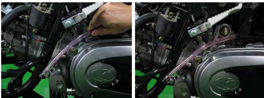
Connect the drain hose from the air box.
