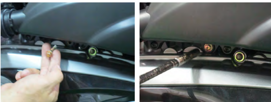
Install the left fender mounting bolts with a 8 mm socket on the front side.
