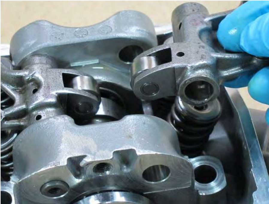
Lift out the rocker arms as the shafts are removed.
