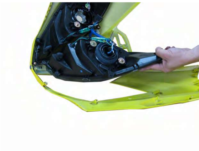
Remove the headlight assembly.
