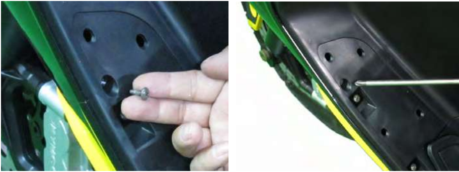
Install the left leg shield mounting screws with a #2 Phillips.
