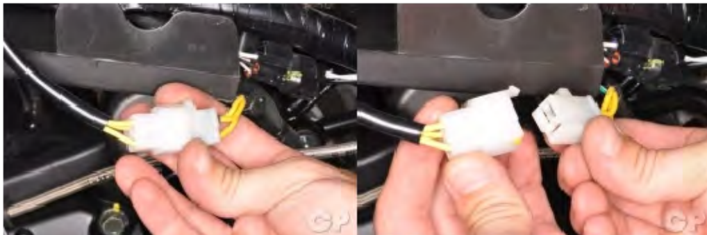
Disconnect the generator 3-pin connector.
