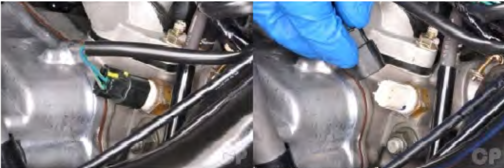
Unplug the water temperature sensor.
