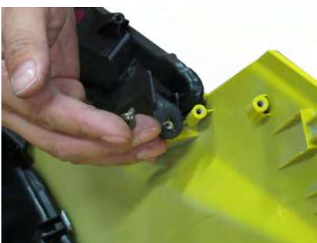
install the turn signal light assembly screws from the front cover.
