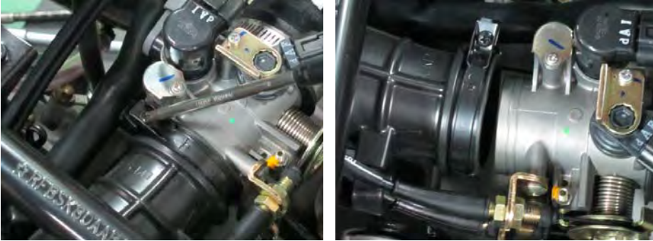
Loosen the air box hose clamp screw at the throttle body with a #2 Phillips.
