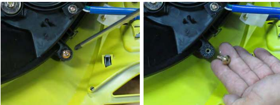
Remove the headlight assembly screws from the front cover.
