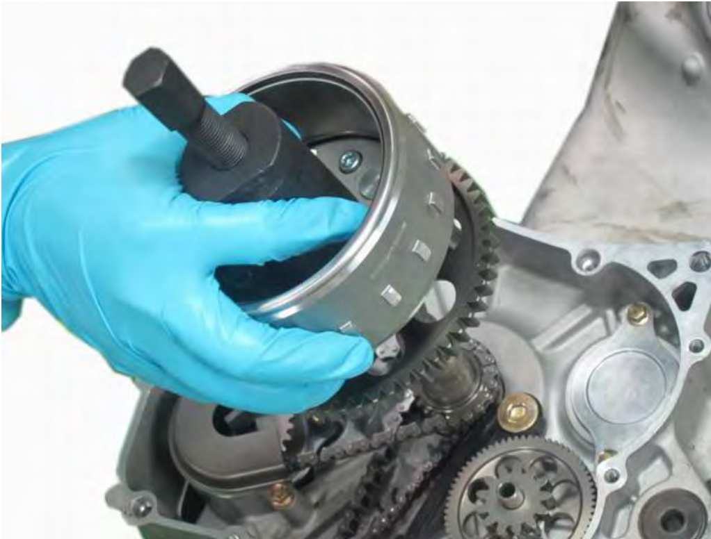
Remove the flywheel from the crankshaft.
