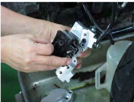
Free the brake pads from the pad retainer. Remove the brake pads.
