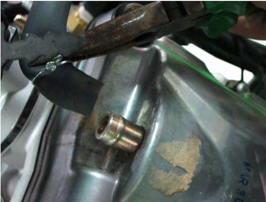
Connect the blow-by tube mounting the cylinder head with a splicer.
