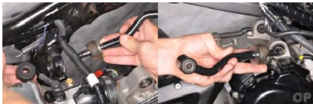
Remove the engine mounting bracket damper assembly.
