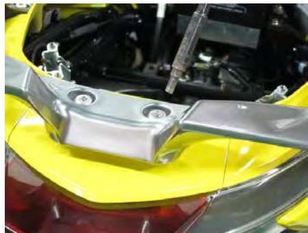
Install the two upper carrier bolts with a 6 mm Allen.
