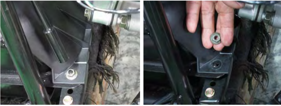
Remove the left fuel tank mounting nuts.
