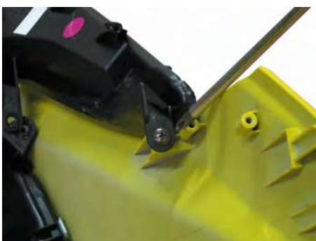
install the turn signal light assembly screws from the front cover.
