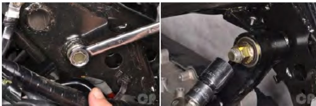
Hold the engine mounting bolts with a 14 mm wrench and torque the nuts to specification with a 19 mm socket.
