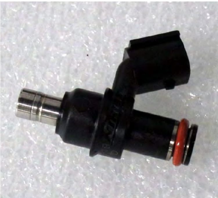
Apply a light coat of fresh engine oil to a new fuel injector O-ring.
