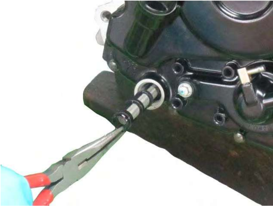
Remove the oil strainer screen.
