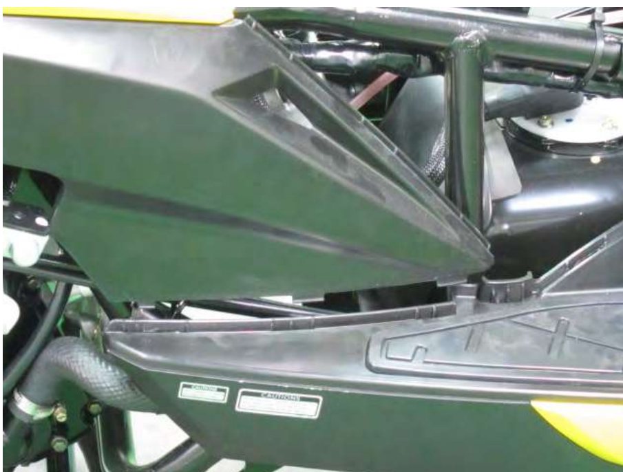
Carefully unhook the tabs on both sides of the body cover.
