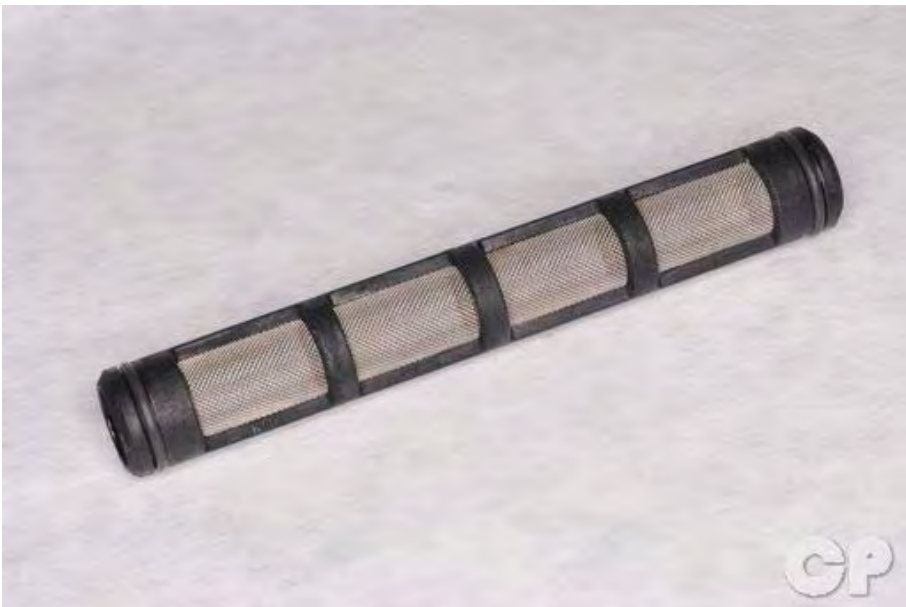
Remove the oil strainer screen.
