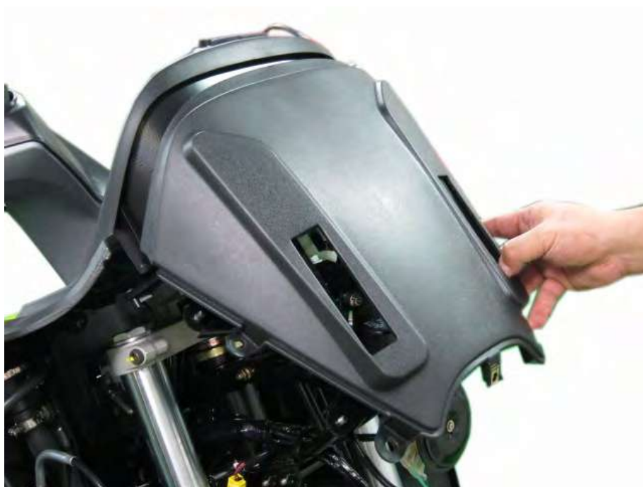
Install the front cover meter
