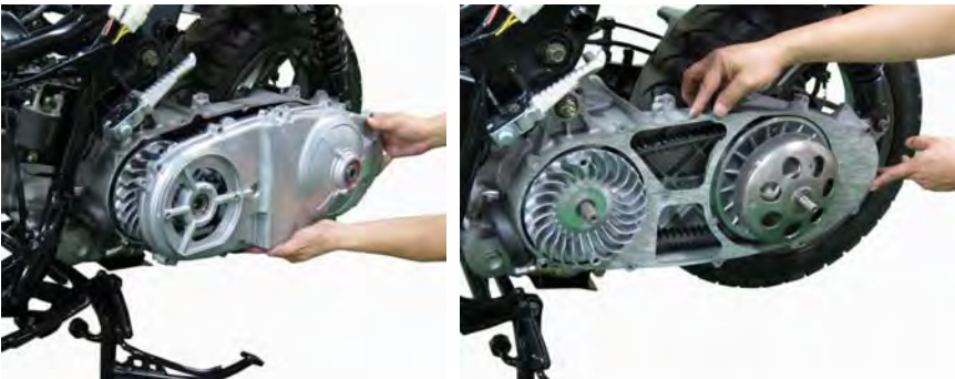
Remove the belt case cover and gasket.
