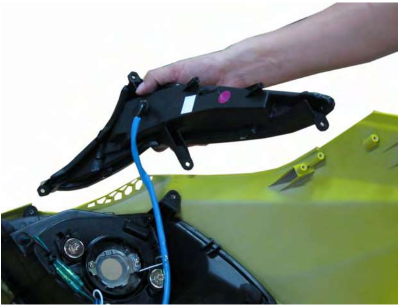
Remove the turn signal light assembly.
