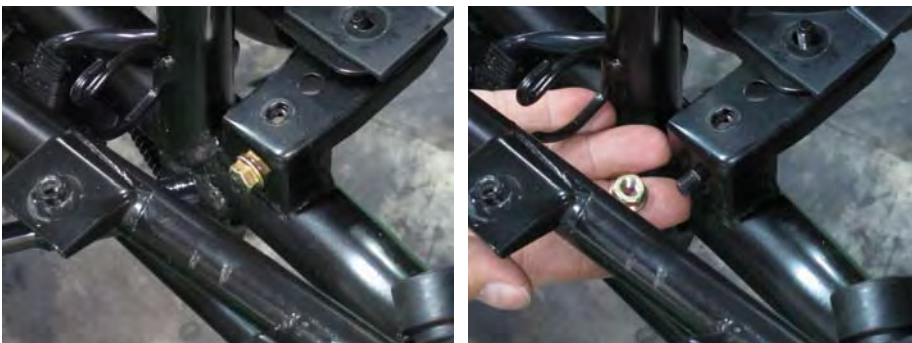
Remove the left fuel tank mounting bolts and brackets.
