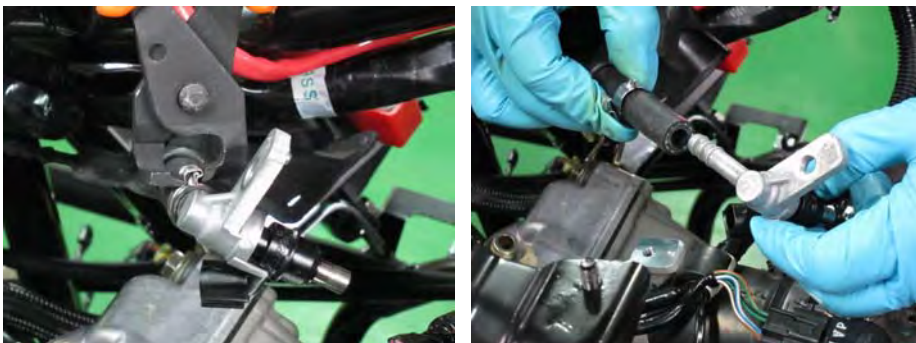
Loosen the fuel hose clamp with a special tool A120F00030. Slide back the clamp and free the injector fuel pipe from the fuel hose.
