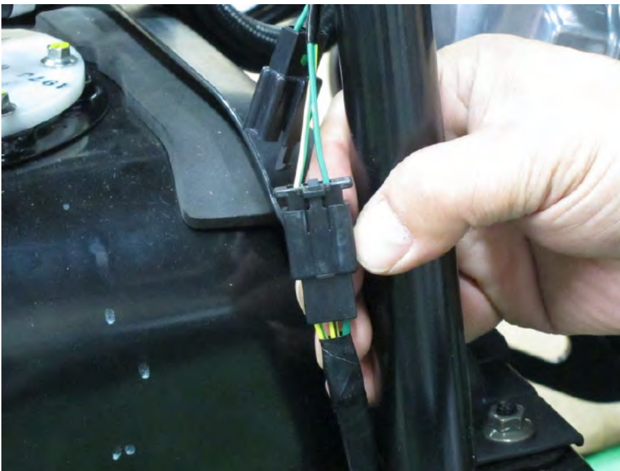
Unplug the three-pin side stand switch connector.
