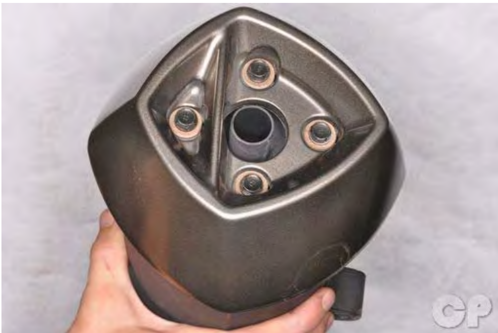
To remove the four bolts to free the heat shield on the muffler.
