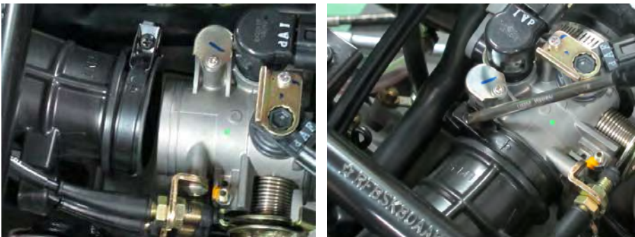
Install the screw mounting the connecting tube airbox.
