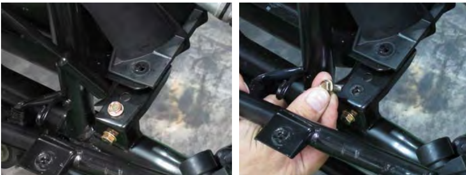
Remove the left fuel tank mounting nuts.
