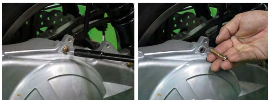
Remove 11 the belt case cover bolts with an 8 mm socket.
