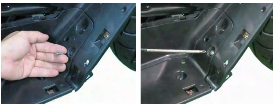
Install the mounting screw with a #2 Phillips on right side.
