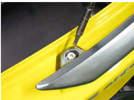
Install the two carrier bolts on each side with a 6 mm Allen.
