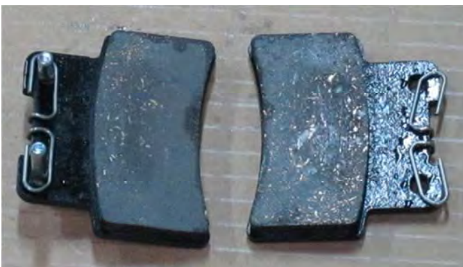
Replace the pads if the brake wear exceeds the wear indicator lines or if the wear is uneven. Always replace brake pads as a set.
