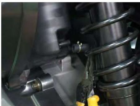
Connect the blow-by tube mounting the transmission box assy.
