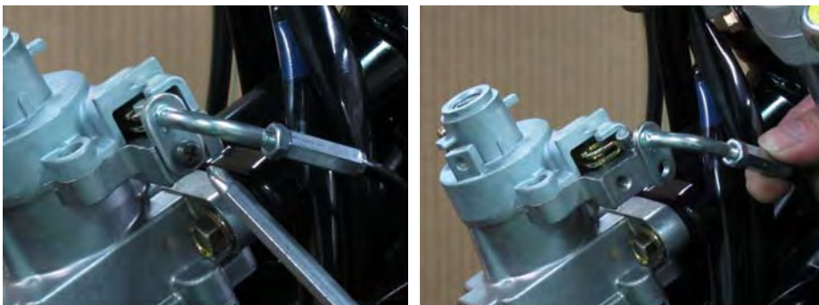
Remove the seat latch cable screw and free the seat latch cable from the ignition switch.
