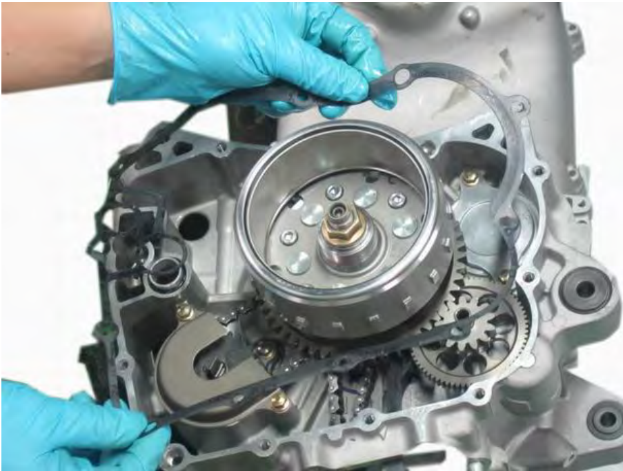
Remove the generator cover gasket.
