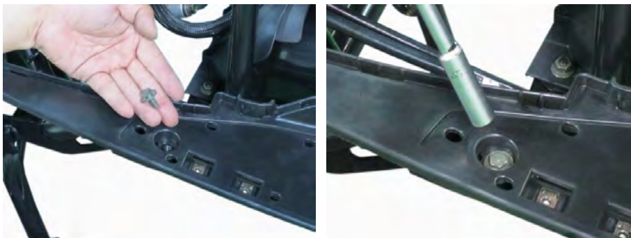
Install the three mounting bolts on right side with a 10 mm socket.
