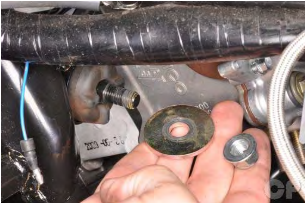
Install the engine mounting bracket damper washer and nut.
