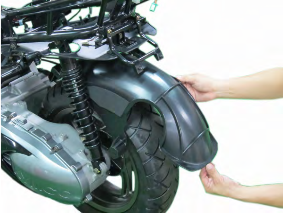
Install the rear fender.
