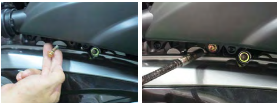
Install the two air box bolts and tighten securely with an 8 mm socket.
