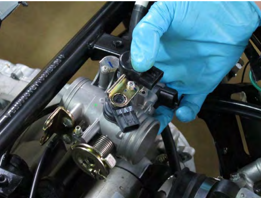
Remove the throttle out of the air box and intake boots.
