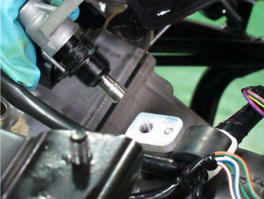
Lift the fuel injector out of the intake pipe.
