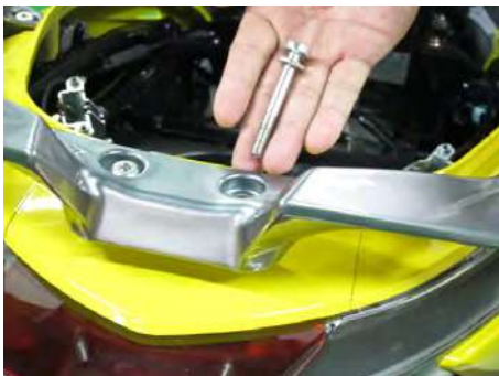
Install the two upper carrier bolts with a 6 mm Allen.
