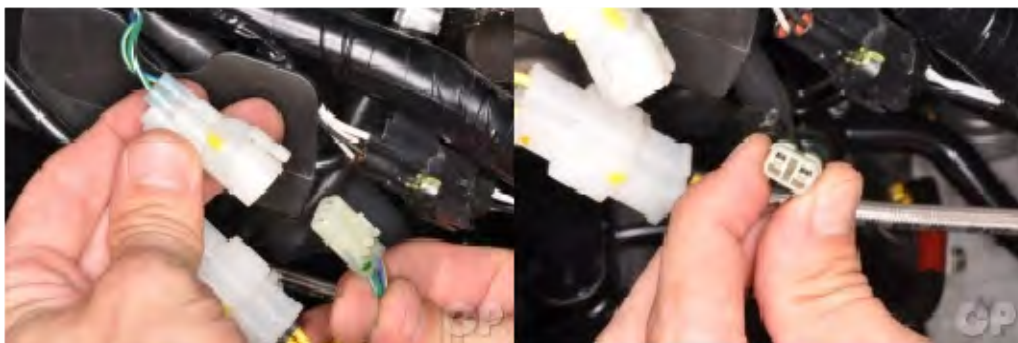
Disconnect the crank position sensor wire coupler.
