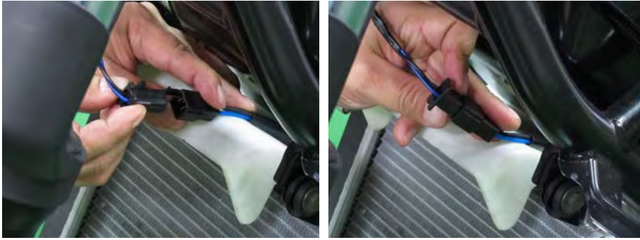
Plug in the cooling fan motor connector.
