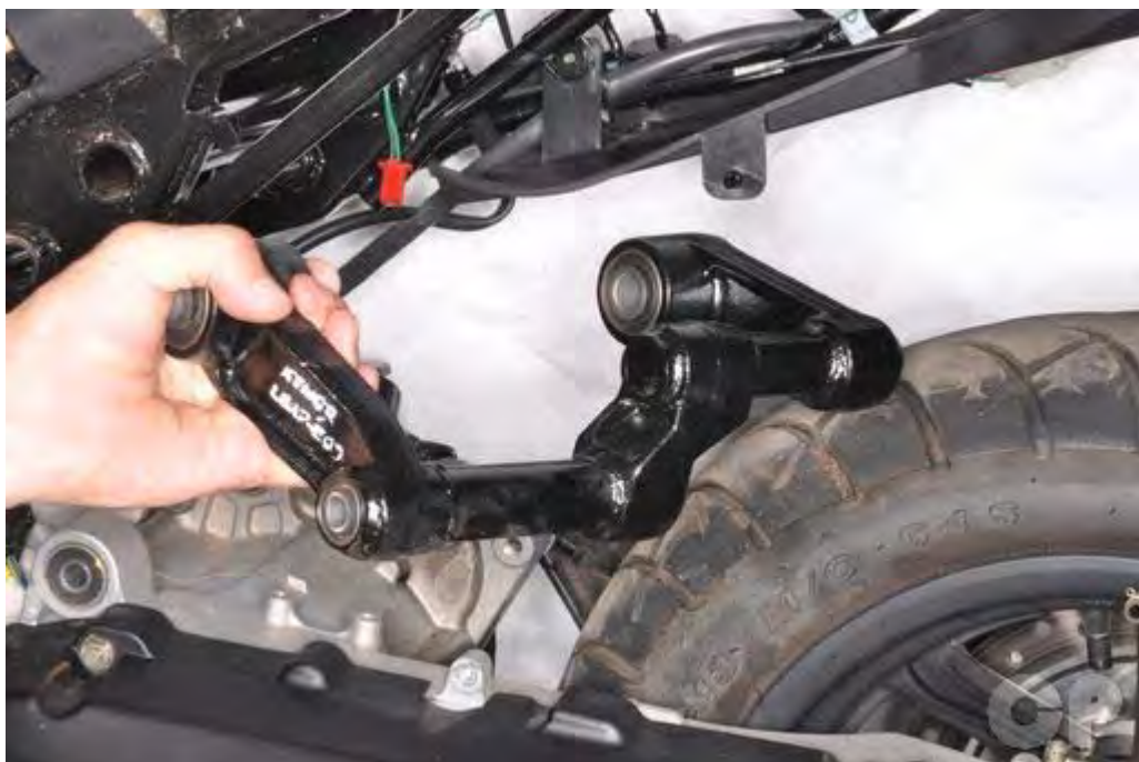
Remove the engine mounting bracket.
