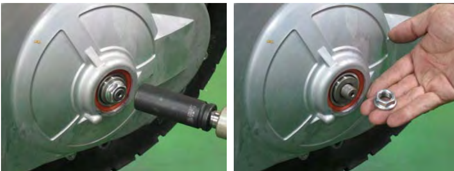
Remove the driven pulley nut with a 24mm socket.
