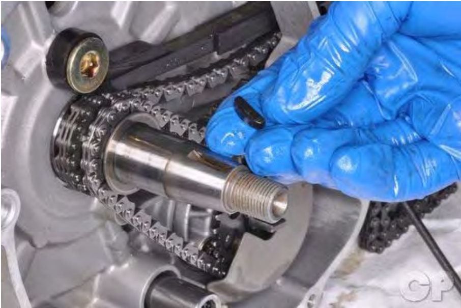
Remove the woodruff key from the crankshaft.
