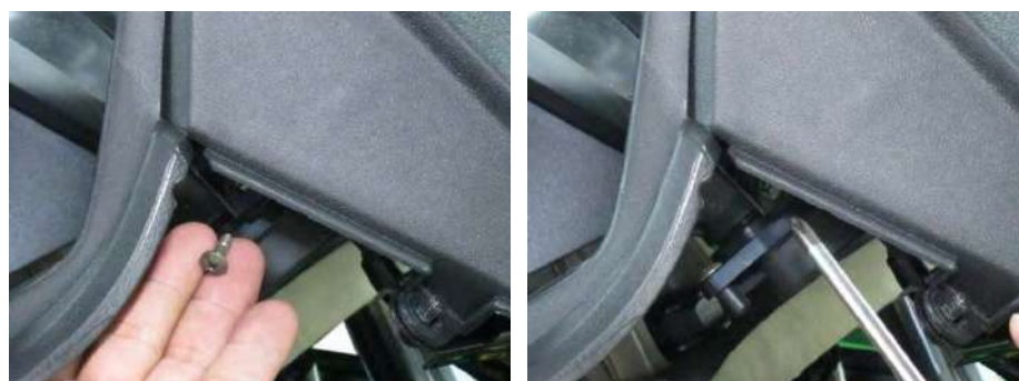
Install the two screws mounting on the front cover meter on both side.
