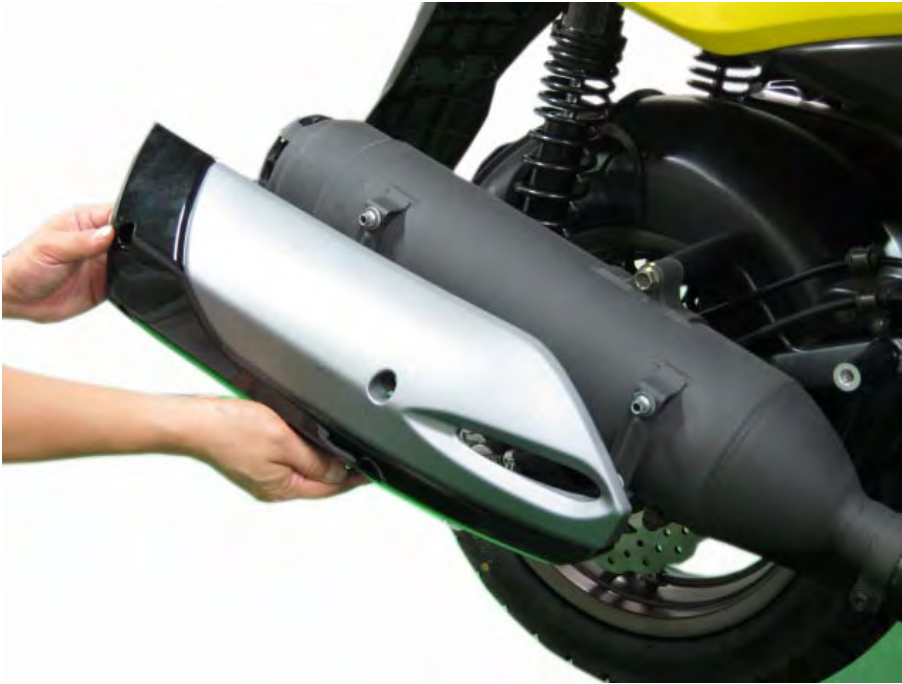
Remove the heat shield.
