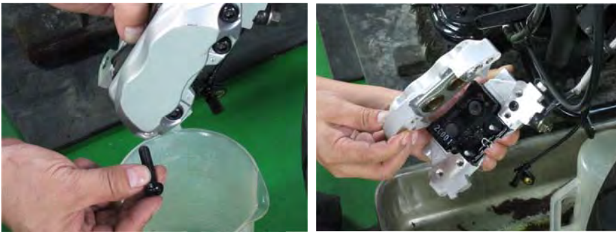
Remove the brake pads with a 6mm Allen.
