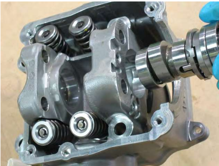
Remove the camshaft from the cylinder head.
