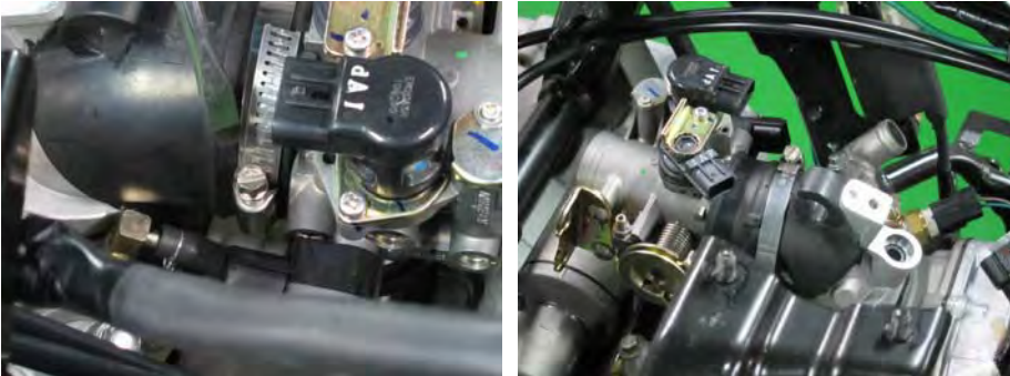
Loosen the intake hose clamp screw at the throttle body with a flat blade screwdriver.
