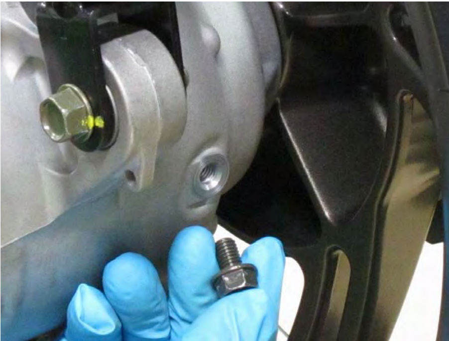
Thread in the final drive oil level check bolt.
