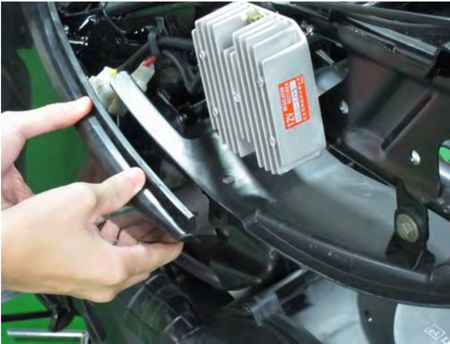
The regulator/rectifier is located on the right side of the vehicle.
