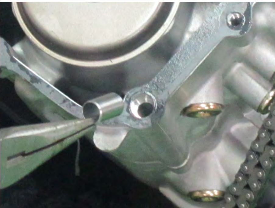
Remove the two dowel pins.
