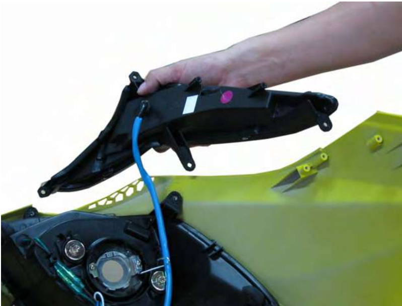
Install the turn signal light assembly.
