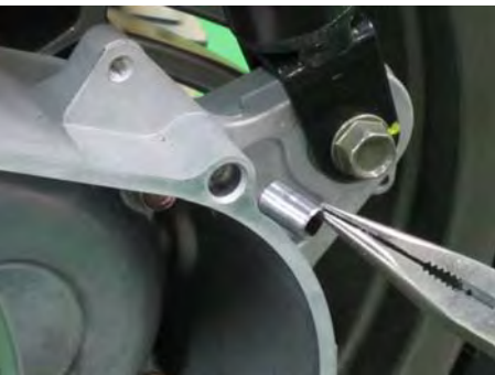
Remove the two dowel pins.
