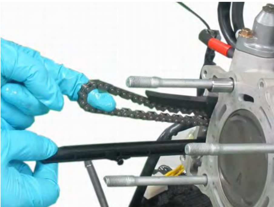
Insert the lower cam chain guide and make sure it is seated correctly.
