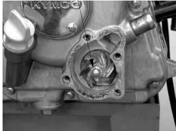
Impeller (Left Hand Threads)
