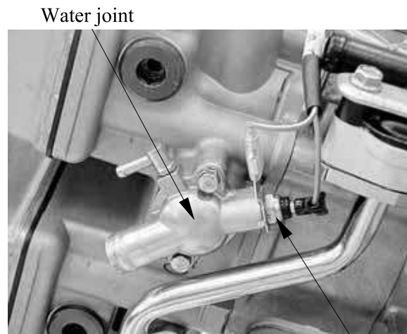
Water Temperature Sensor
