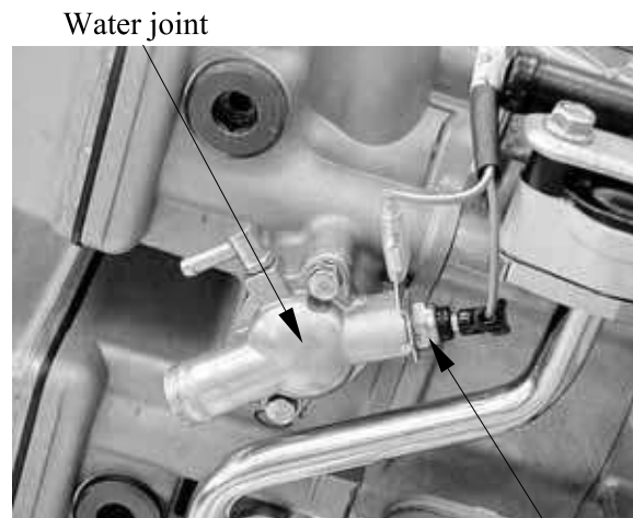
Water Temperature Sensor
