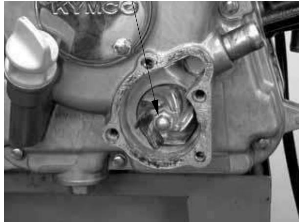
Impeller (Left Hand Threads)
