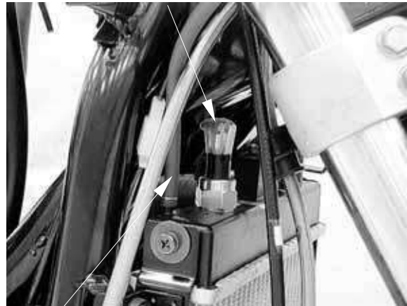
Air Bleed Hose
