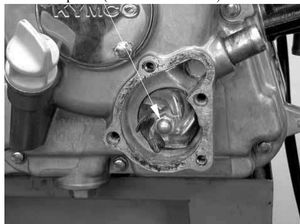
Impeller (Left Hand Threads)
