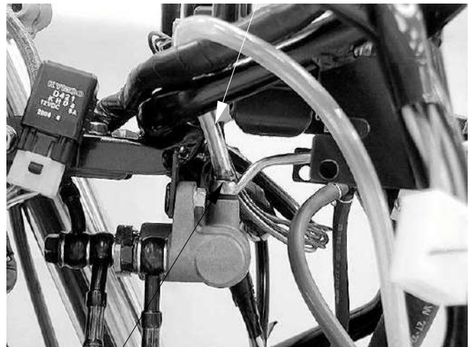
Relay Valve Air Bleed Screw
