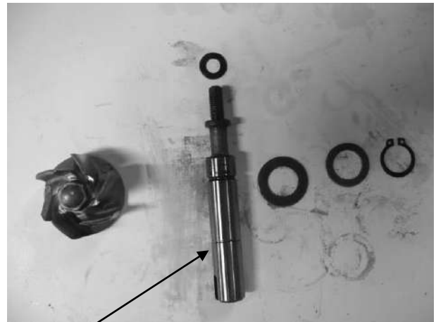
Water pump shaft
