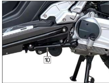
7. Side (10) switch at horizontal position.
