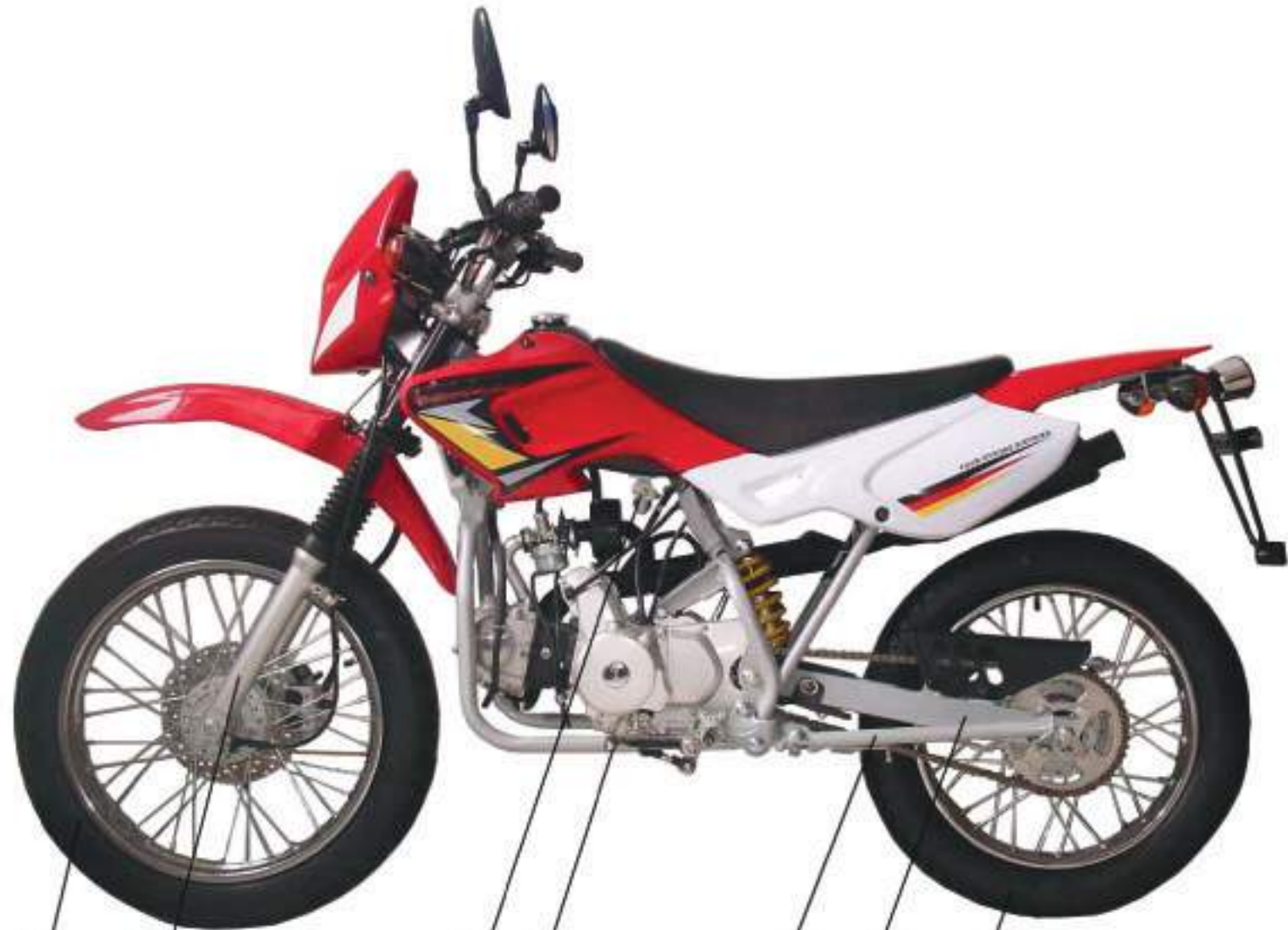
1. front wheel 2. front shock absorber 3. fuel cock 4. gear shifting 5. side stand 6. rear fork 7. rear wheel
