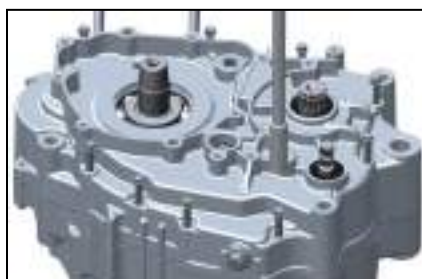
Mount the mould closing bolt
