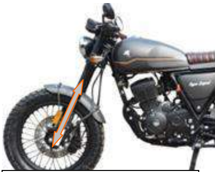
Front suspension inspection
